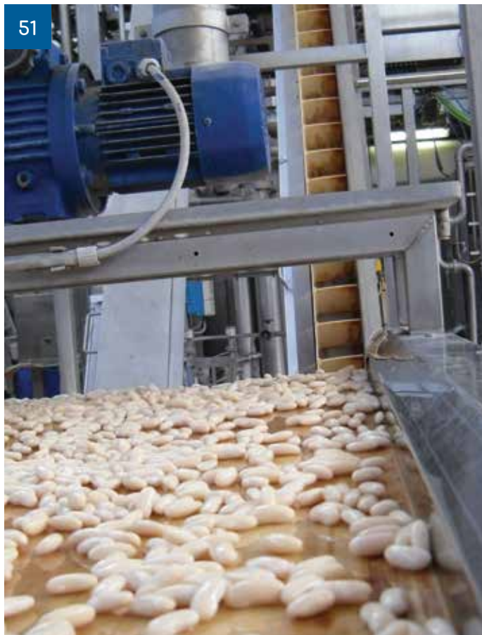
Cooked Beans on SD™ Bead Elevator
