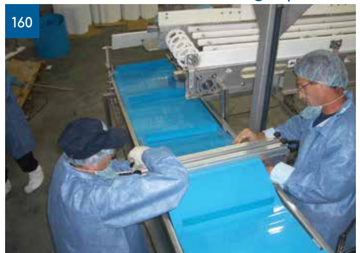
On-site Installation with Volta FBW - Flat Butt- Welding System
