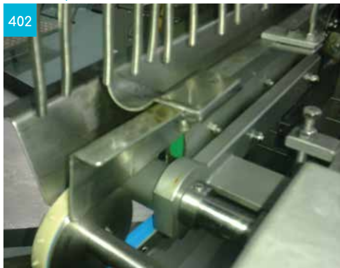
Apple Washing - RL Profile Used as Agitator
