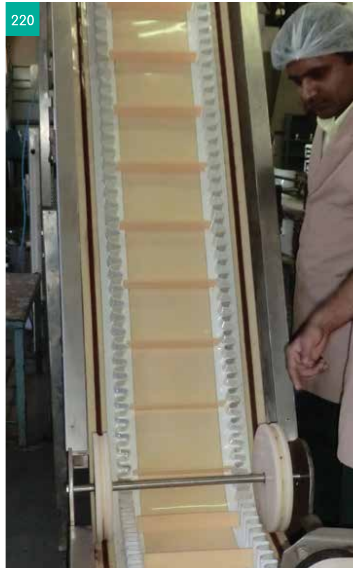
New - Volta Belt After 18 Months
