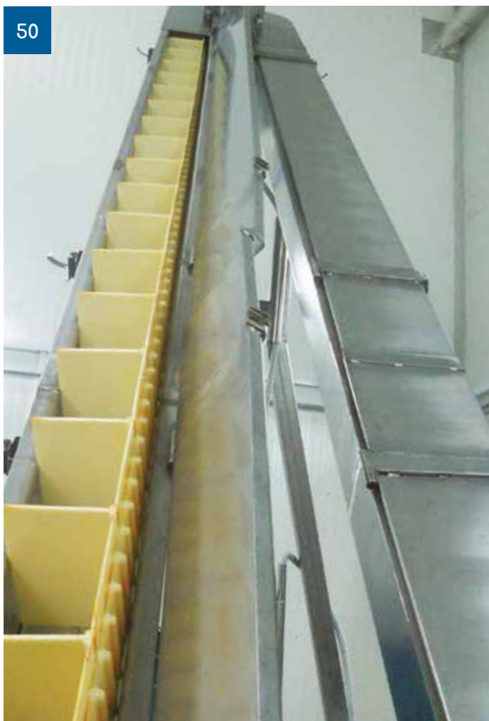
Cooked Beans on SD™ Bead Elevator
