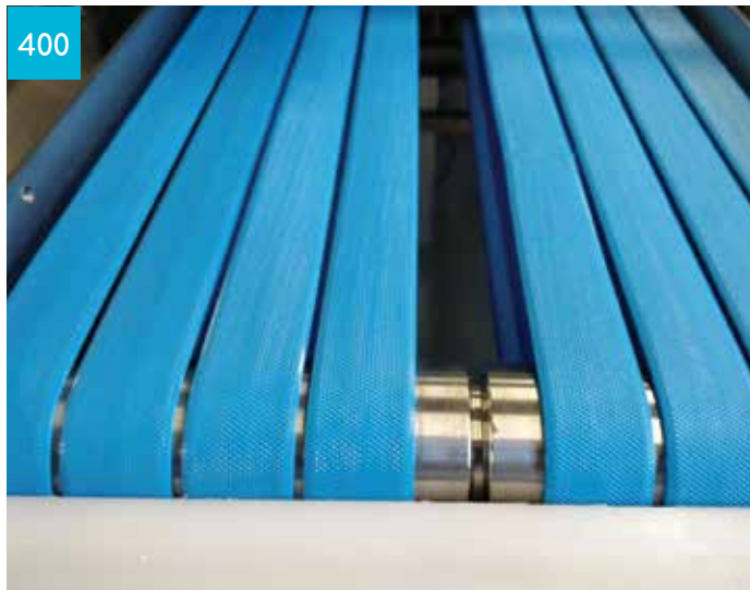
Fish Conveying VMW with Spike Texture
