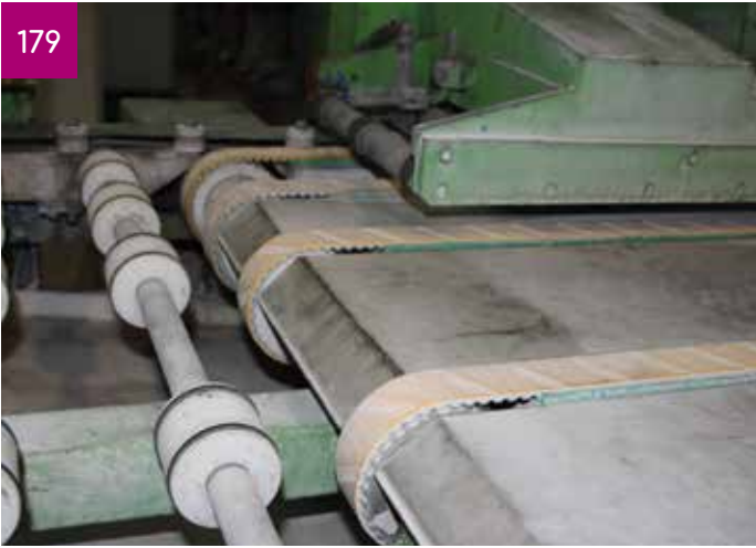
Machined FMB Belt with Grooving Welded on Timing for Glass Conveying
