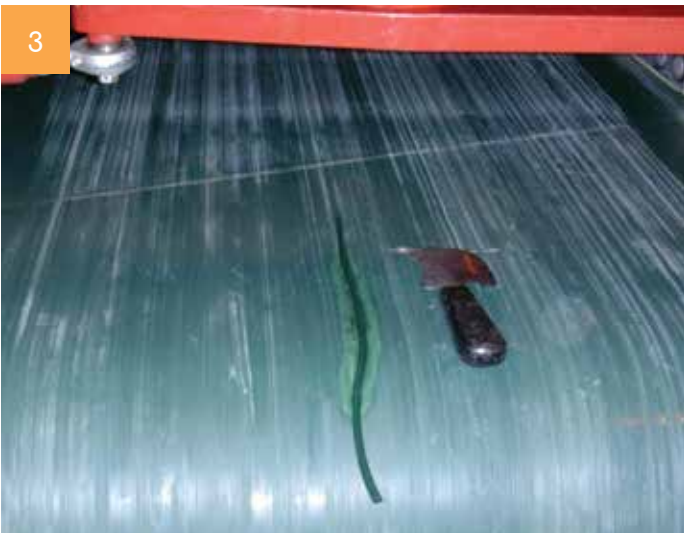
FRPZ-8 belt repaired with electrode
